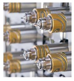
UltraSync technology allows for close nozzle spacing.
